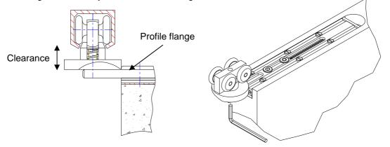
The clearance between hanger and collar should allow the collar to slide without problem on the profile flange unhindered. While the door leaf set is closing the collar rotates. The slope at the collar enables to slide on top of the profile flange.
